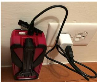
If the battery is flat, insert the adapter into the receptacle at the end of the radio and then plug the other end into a USB outlet in a plug. See the photo. The adapters for the radios given out before mid 2017 plug directly into a wall outlet and take several hours to recharge. (I left mine overnight.) The newer radios can also be recharged by plugging them into the USB port of any device with a charged battery, such as a computer, laptop or USB car lighter adapter.
